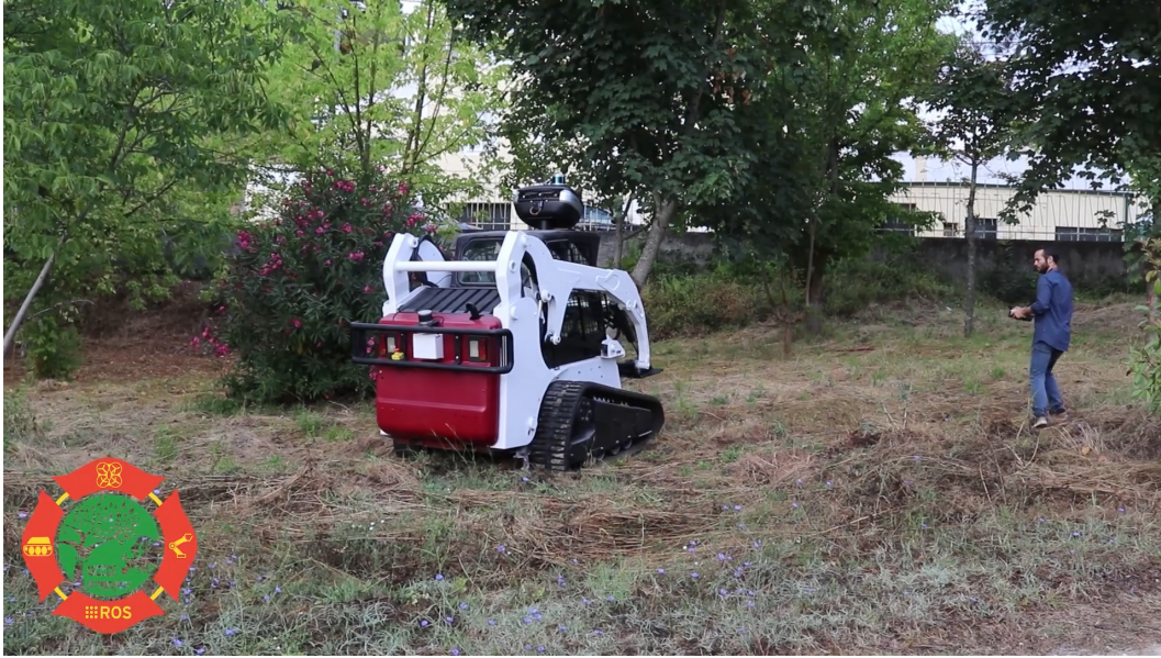
Figure 18: Ranger’s remotely controlled experiment in the field. Full video available at: https://www.youtube.com/watch?v=Jo99beTU2J8 .
