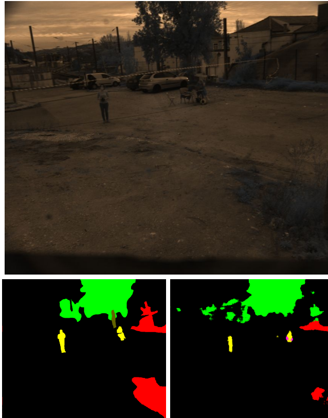
Figure 36: Semantic segmentation results in our experimental setup. Original multispectral image on top; Ground truth on the bottom left, prediction on the bottom right. Colors are yellow for humans, red for fuel, green for canopies, brown for trunks and purple for animals.
