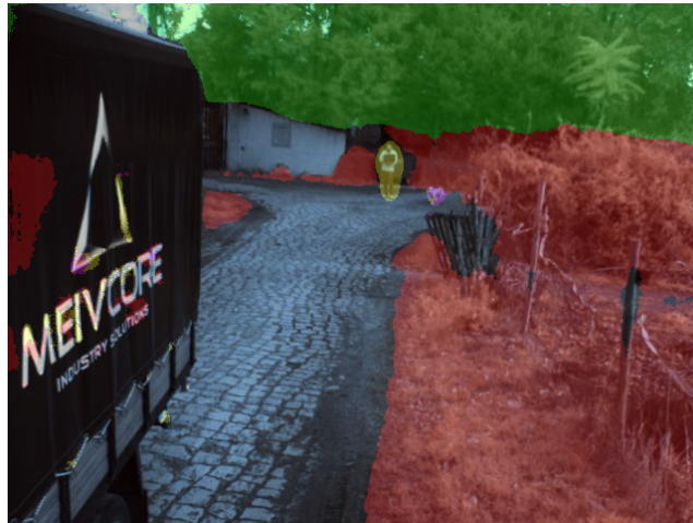
Figure 33: Example of ground truth (left) and respective prediction (right) made by MobileNetv2 backbone and ASPP progressive decoder with fine tuning showing mislabeling of features on the side of the truck as being member of other than the expected Background class.
