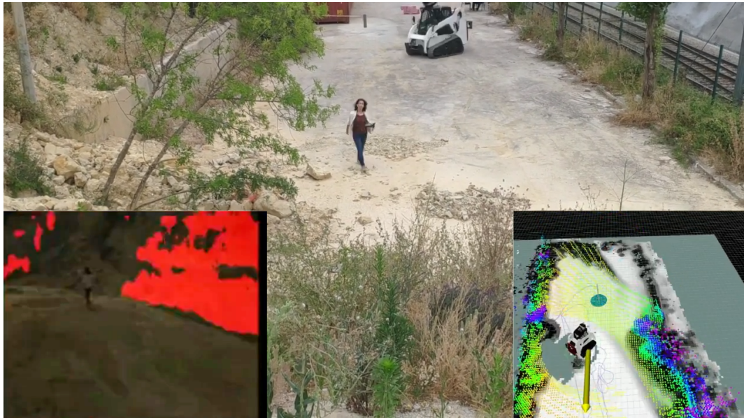
Figure 22: Combined Traversability Analysis and Image Segmentation.
