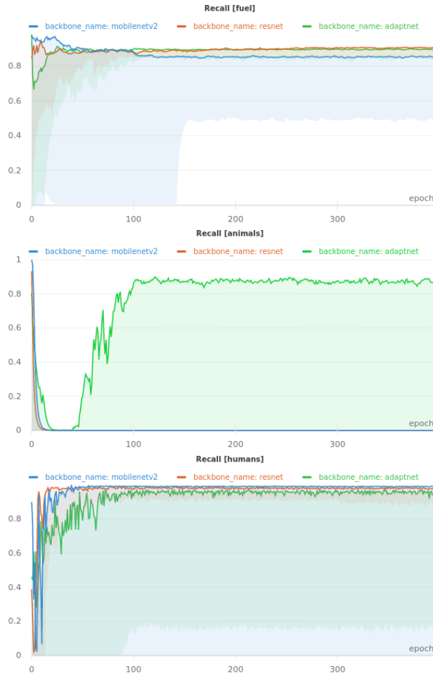
Figure 31: Comparison plots of Recall vs Epoch for the Adaptnet++ , ResNet50 and MobileNet encoders, for the Fuel, Animals and Humans classes resulting from the sweep made using Weights and Biases (respectively, from top to bottom). Coloring scheme follows same convention as with Fig. 30.
