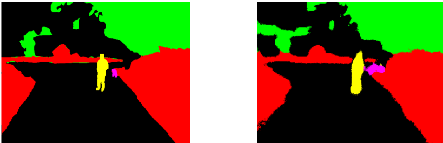
Figure 29: Example output for model consisting of Adapnet++ backbone, eASPP progressive decoder and fine tuning trained on Bonnetal using Imagenet pre-weights for the whole model. Ground truth image is shown on the left and corresponding prediction on the right.
