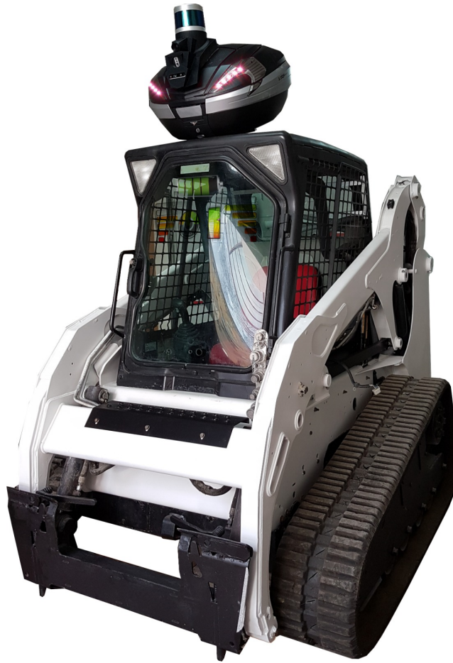
Figure 2: The Ranger platform without the mulcher attachment. The platform is based on the Bobcat T190, and is being equipped with a sensor and computational array, using the black box at the top.
