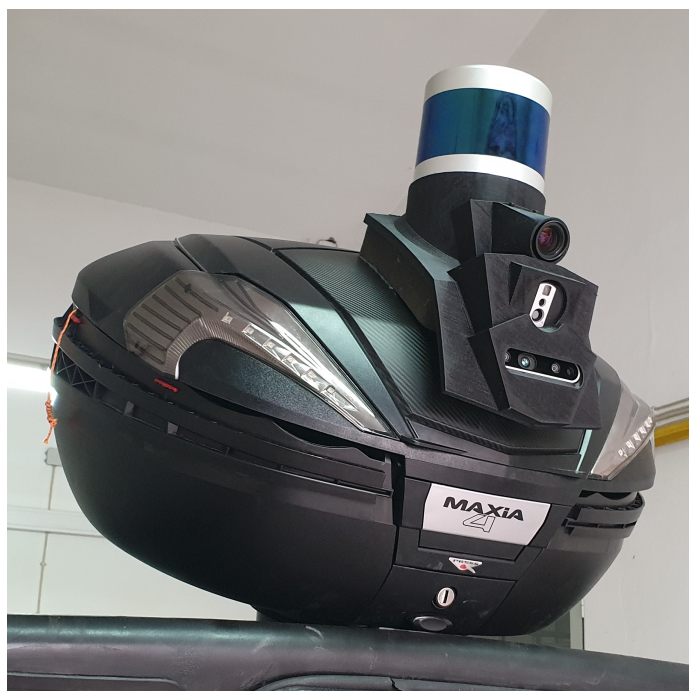
Figure 3: Close-up of a preliminary version of the main sensor array installed on the Ranger. Visible sensors, from top to bottom: LeiShen C16, Genie Nano C2420, FLIR AX8, and RealSense D415.
