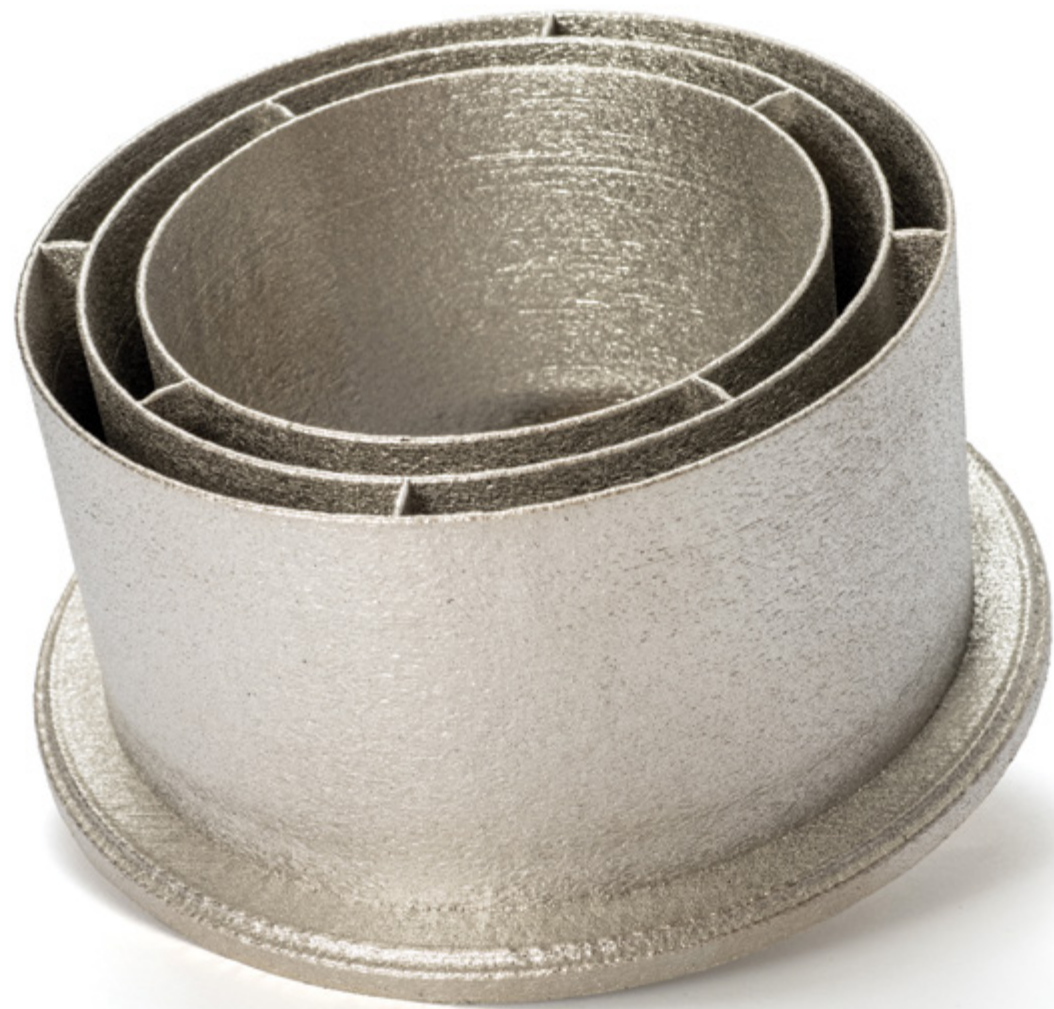
A magnetic shield created with blown powder laser deposition.
