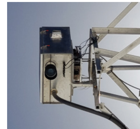
A view of the camera box as attached to the tracking dish.
