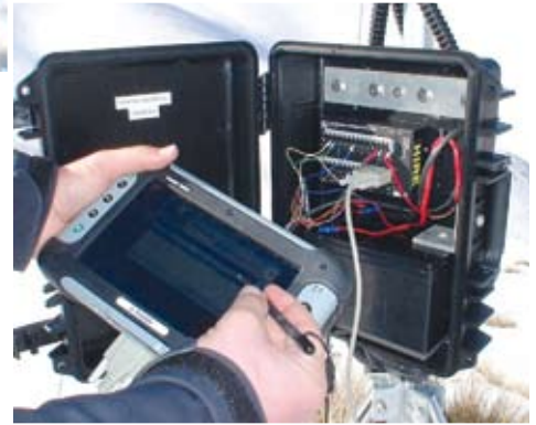
Downloading meteorological data from one of the Crystal Valley automatic weather stations with the Trimble rugged tablet computer (close up, right).
