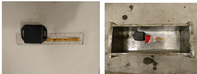
Figure 2-3. Packaging concept to engage concrete in embedded applications.
