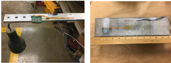
Figure 2-2. RFID and wired strain gauges installed on the surface of Aluminum cantilever the concrete beam.
