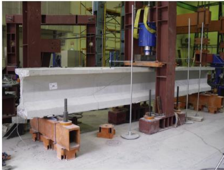
Fig. 5. Beam during shear test.
