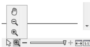
Figure 2.15: Additional mouse modes can be found in the zoom tools when right-clicking on the magnifying glass.
