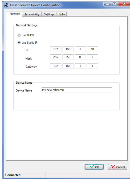
Figure 9: Kvaser Remote Device Configuration network settings
