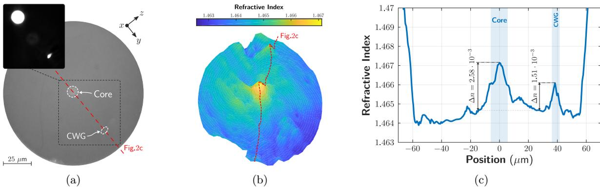
Figure 2. (a) SMF end-face of the inscribed waveguide captured with a CCD camera, along with the output light obtained when a white light source is connected to the distal end of the fiber sample. (b) 3D RI profile measured with a Refractive Index Profiler. (c) Core and CWG RI profile.
