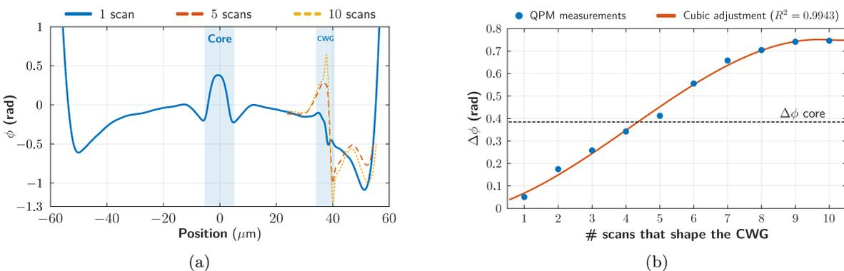
Figure 3. (a) Phase profile measured with QPM for waveguides inscribed by 1, 5 and 10 scans, (b) and the CWG-cladding phase change based on the number of scans that form the waveguide.
