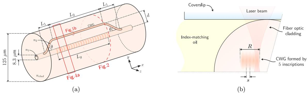
Figure 1. (a) Dimensions of the all-in-fiber 6 mm component formed by the MZI and the FBG located in the core, with references to the figures containing the CWG-FBG inscription result, the CWG cross-section, (b) and the multiple inscriptions used in the manufacture of the CWG (cladding section of the MZI).
