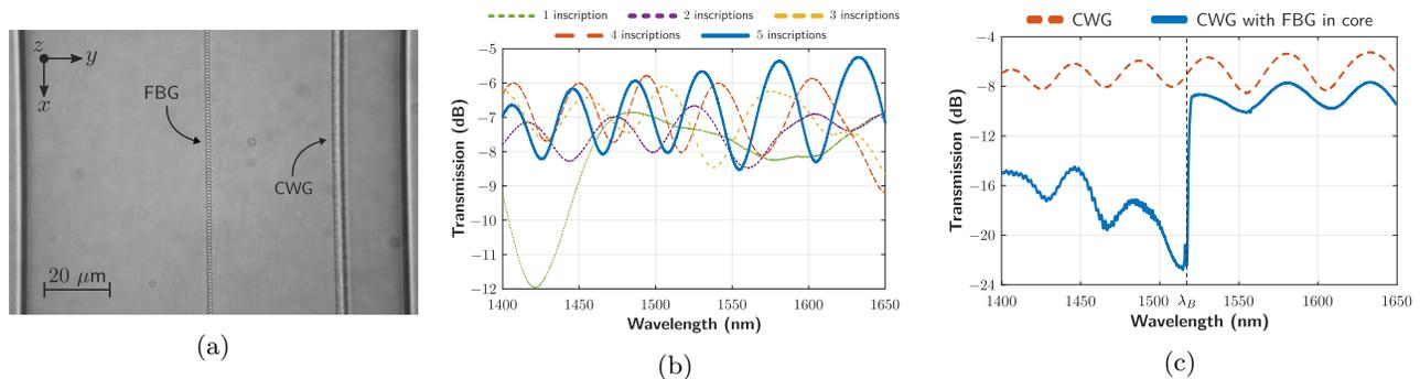
Figure 4. Manufacturing result. (a) Longitudinal view of the MZI cladding section together with the FBG inscription in the core. (b) MZI transmission spectra for waveguides formed between 1 and 5 scans, (c) and a comparison of the transmission spectra of the complete MZI (5 scans) without and with the FBG in the core.
