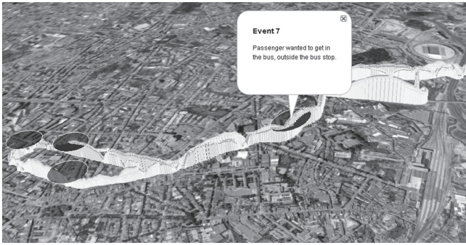
Fig. 4. Visualization of a trip and stress events in Google Earth. The height of the traces represents bus speed, ellipses denotes events.
