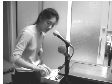
Figure 2. A player records her singing voice and manipulates it by moving her finger over the touch pad
