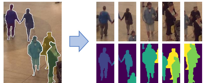
Fig. 6. Multiple export formats exist, among which is a utility that crops components out of the image, optionally padding with scene pixels and resizing to ensure all shapes are equal. Each sub-image and mask is saved accordingly, which is useful for training on multiple forms of machine learning models.
