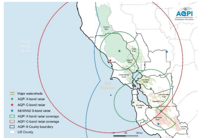
AQPI and NEXRAD radar coverages in the SF Bay Area. Small (large) circles are 40 (150) km coverage rings, and dashed circles indicate NEXRAD coverages.
