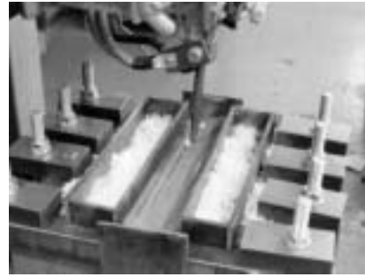
Fig 7 Assembly for testing welds for HICC, with removable clamping and dry ice cooling
