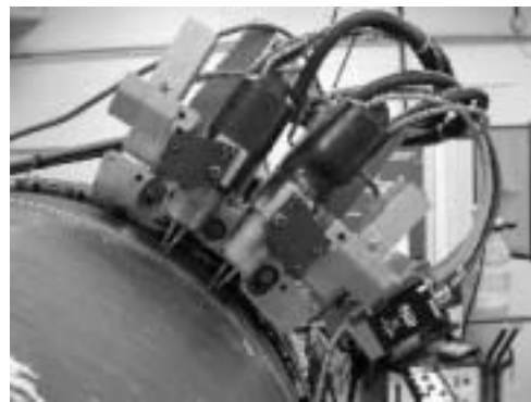
Fig 4: CAPS dual-tandem GMAW torches on RMS welding bug
