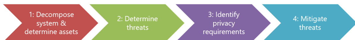
Figure 12. Privacy engineering process based on the security engineering process by Brost and Hoffmann (2015, p. 138).
