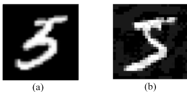
Figure 2: Original image is a digit 5. (a) Natural attack; (b) Unnatural attack (minor changes in pixel values of the background compared to the original). Under both of these attacks, the neural network classifies the image as 3 instead of 5.
