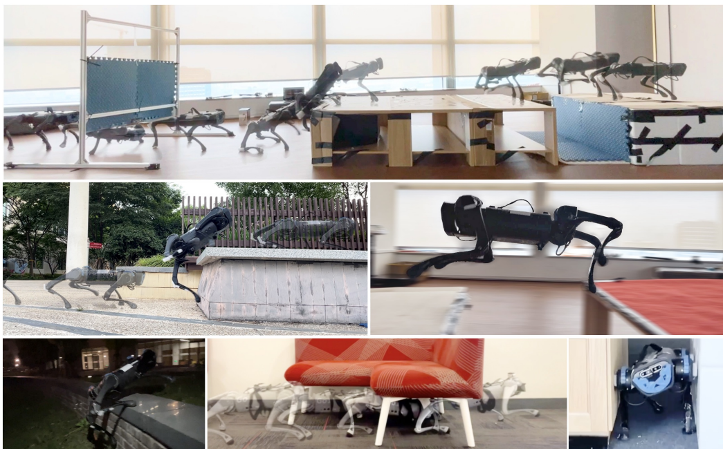
Figure 1: We present a framework for learning parkour skills on low-cost robots. Our end-to-end vision-based parkour learning system enable the robot to climb high obstacles, leap over large gaps, crawl beneath low barriers, squeeze through thin slits and run. Videos are on the project website .
