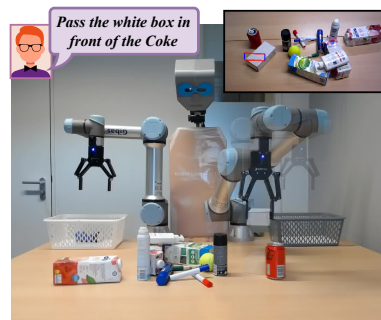
Figure 1: 4-DoF referring grasp synthesis in clutter.
