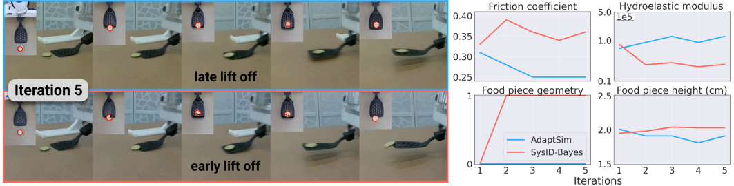
Figure 8: Adaptation in Scooping Task. With AdaptSim, the cucumber is successfully scooped up by lifting up the spatula off the table late; otherwise, the piece slips off the spatula. AdaptSim infers an ellipsoidal shape ( g=1 , food piece geometry), while SysID-Bayes infers a cylindrical shape.
