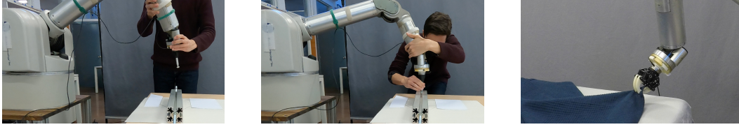
Figure 1: The tasks involved in our experiments. In the first two pictures, the human is guiding the robot to perform: a free motion above a metal piece; the insertion of the end-effector in the trail inside the piece. In the last picture, the robot is pulling a bed sheet to remove the wrinkles.
