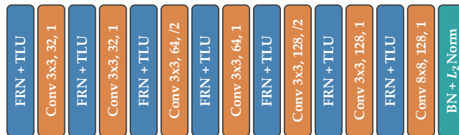
Figure 5: The network architecture is the same as that proposed by HyNet (Tian et al. (2020)) with a dropout rate of 0.3.
