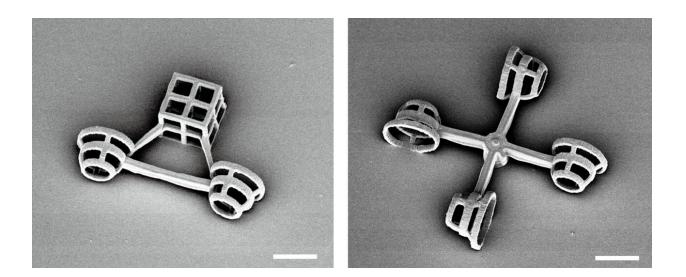
Scanning electron microscope images of the two micromachines: These photos show the "scooter" (on the left) and "rotator" (on the right). Each micromachine was observed in detail and using motion tracking for 70 seconds at a time over several hours. The scale bar length is 10 microns (0.01 millimeter). Credit: *Small* (2024). DOI: 10.1002/smll.202402923
