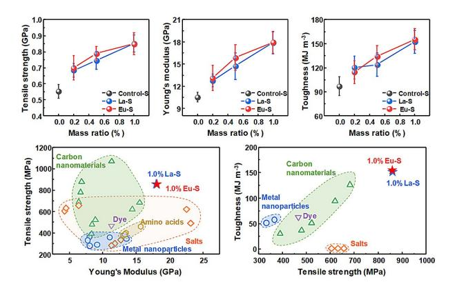
On the above, the strength, modulus, and toughness increased with the mass ration of rare earth ions. On the below, the comprehensive mechanical performance of rare earth ion-modified silk is superior to that of silk modified by other functional materials. Credit: Science China Press
