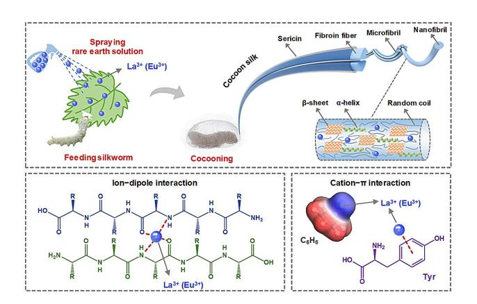
On the above, the rare earth solution was sprayed on mulberry, which was fed to silkworm to spun reinforced silk fibers. On the below, it illustrates the ion-dipole and cation- $\pi$  interaction between rare earth ions and silk. Credit: Science China Press
