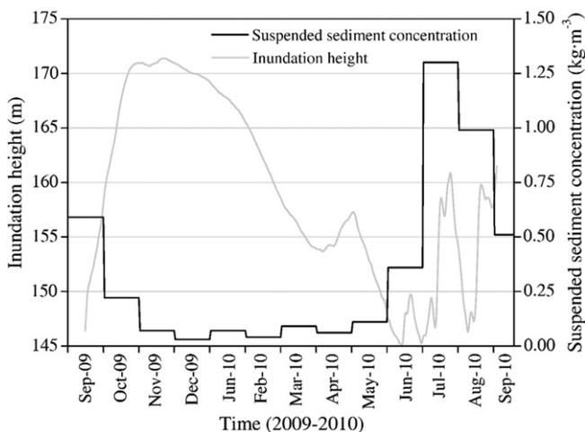
**Fig. 7.** The seasonal variation of monthly average suspended sediment concentrations and water levels during the 2009–2010 hydrologic year.
