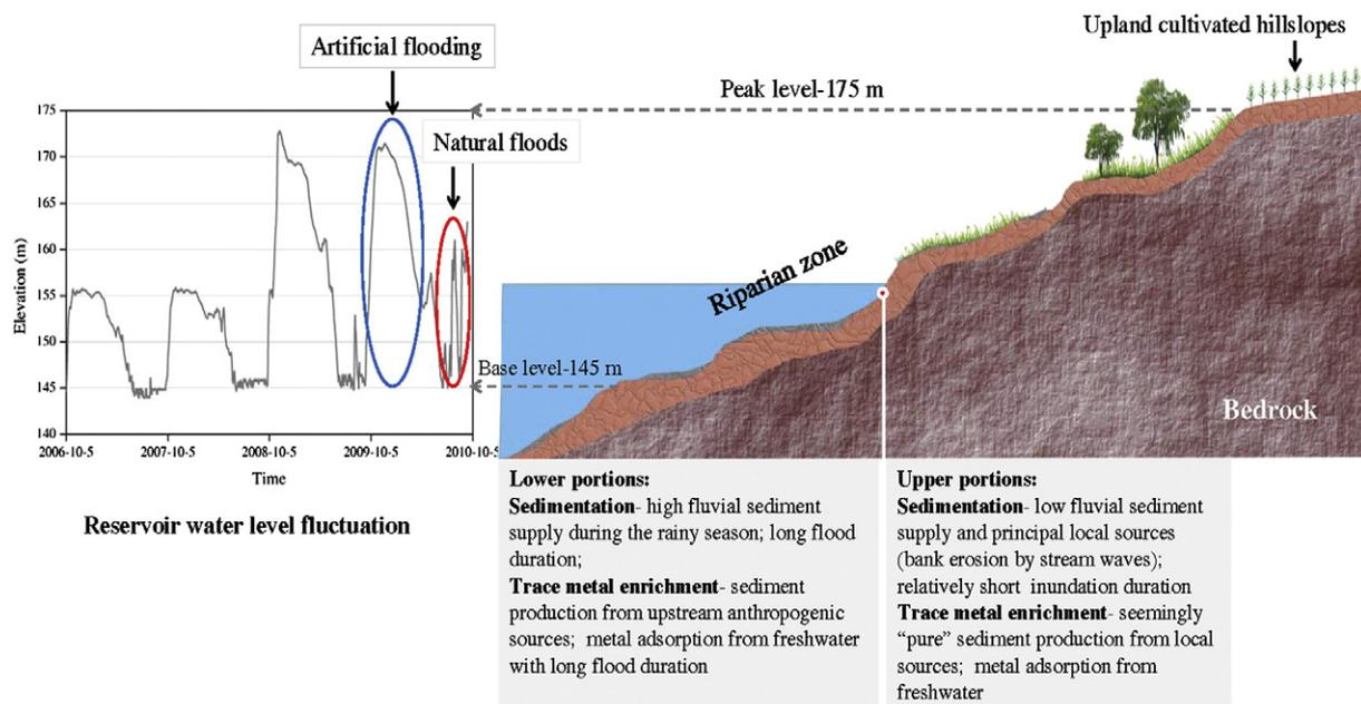
Fig. 2. The changes in water level by regular dam operation since 2006 in the riparian zone, as well as the contrasting processes of sedimentation and trace metal enrichment at different portions of the riparian zone were illustrated.
