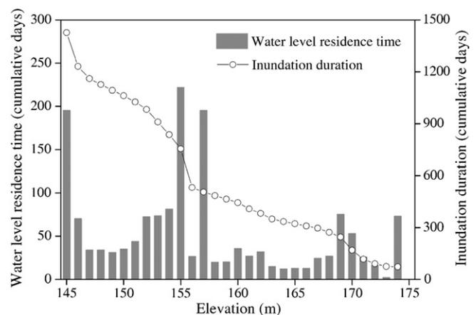
**Fig. 8.** The variation of water level residence time and inundation duration with elevation in the riparian zone.
