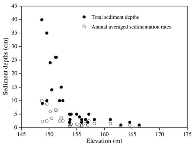
**Fig. 4.** The observed variation of the total sediment depths and annual average sedimentation rates with elevation in the riparian zone.
