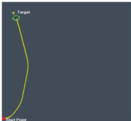
Figure 9: Scenario 1: robot navigation without Obstacle using FLC.
