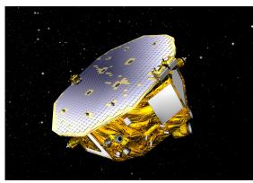
Artist's impression of the LISA Pathfinder spacecraft. LISA Pathfinder will test in-flight the concept of low-frequency gravitational wave detection by putting two test masses into near-perfect gravitational free-fall while controlling and measuring their motion with unprecedented accuracy. Credit: ESA
