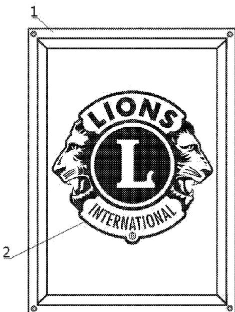
(57) Abstract: Illuminated advertising panel composed of a translucent main panel and a front panel, between which panels there is the signage to be displayed and at least two bands of LEDs each arranged in a recess in the main panel, between which there is a section of diffuser elements.
