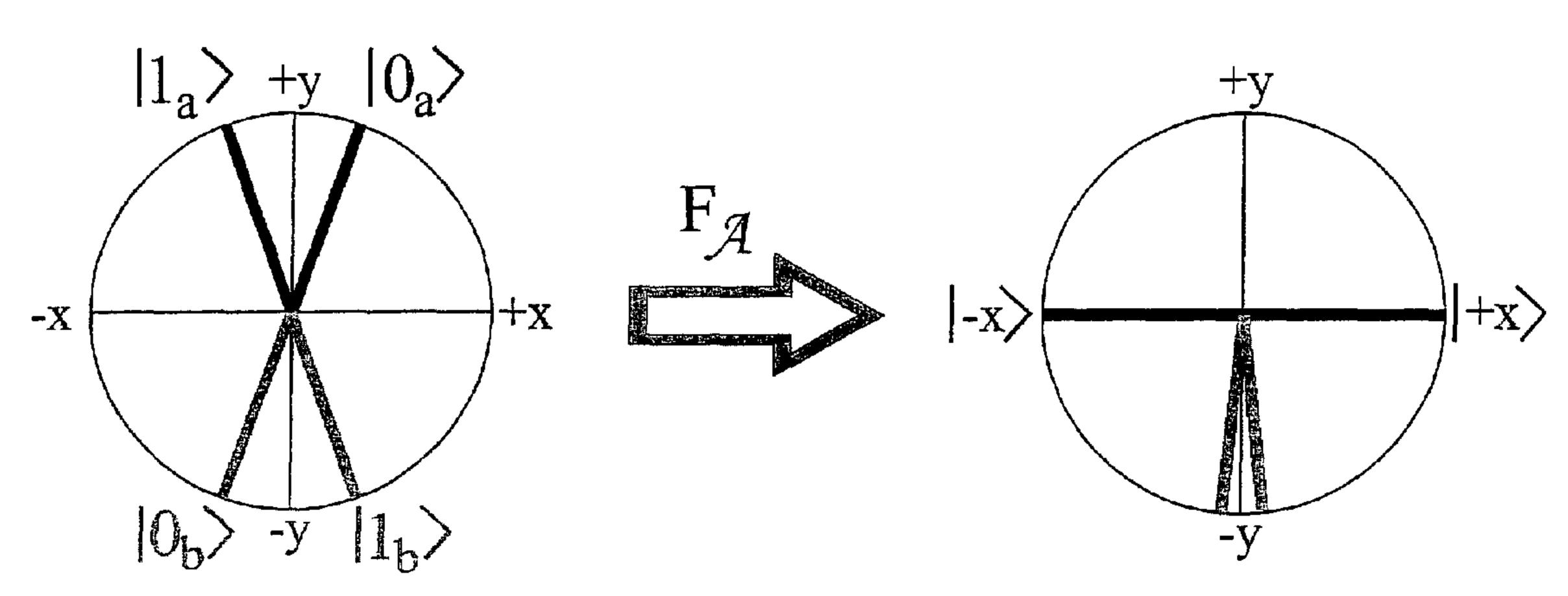
(57) Abstract: An apparatus and method for implementing a quantum cryptography system encoding bit values on approximations of elementary quantum systems with provable and absolute security against photon number splitting attacks. The emitter encodes the bit values onto pairs of non-orthogonal states belonging to at least two sets, and such that there does not exist a single quantum operation allowing to reduce the overlap of the states in all the sets simultaneously.
