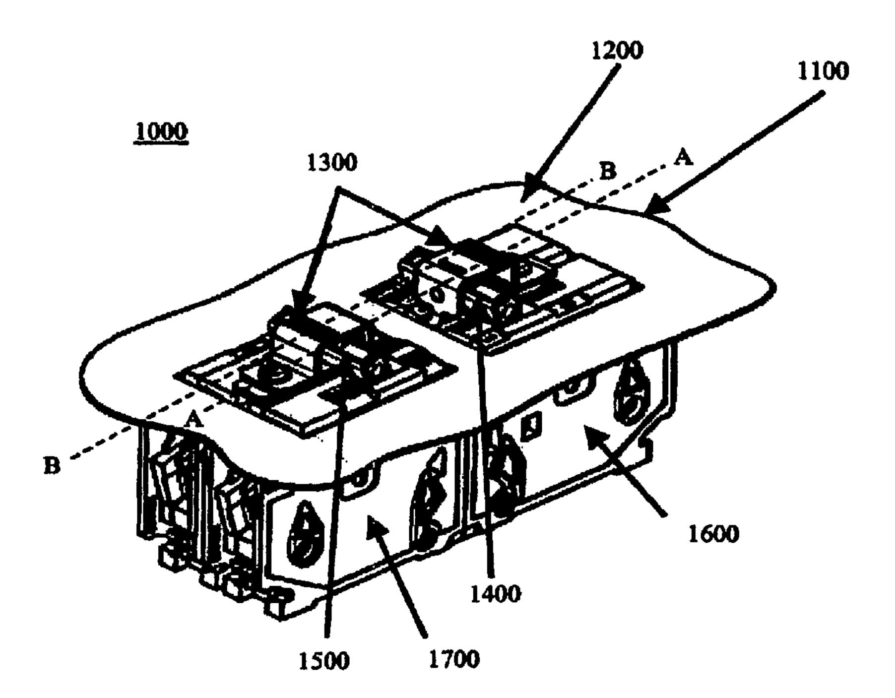
(57) Abstract: Certain exemplary embodiments comprise a breaker interlock device adapted to mechanically resist switching a handle of a first circuit breaker from an OFF position to an ON position when a handle of a second circuit breaker is in an ON position, wherein the first circuit breaker is adjacent to the second circuit breaker.
