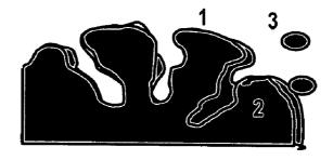
1. Uncoated surface; 2. Plugged Pores; 3. Free Particles
