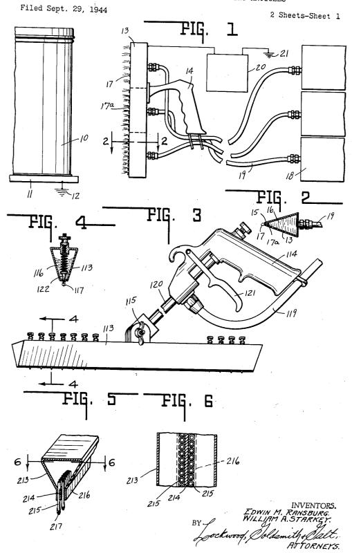
METHOD FOR ELECTROSTATICALLY COATING ARTICLES
