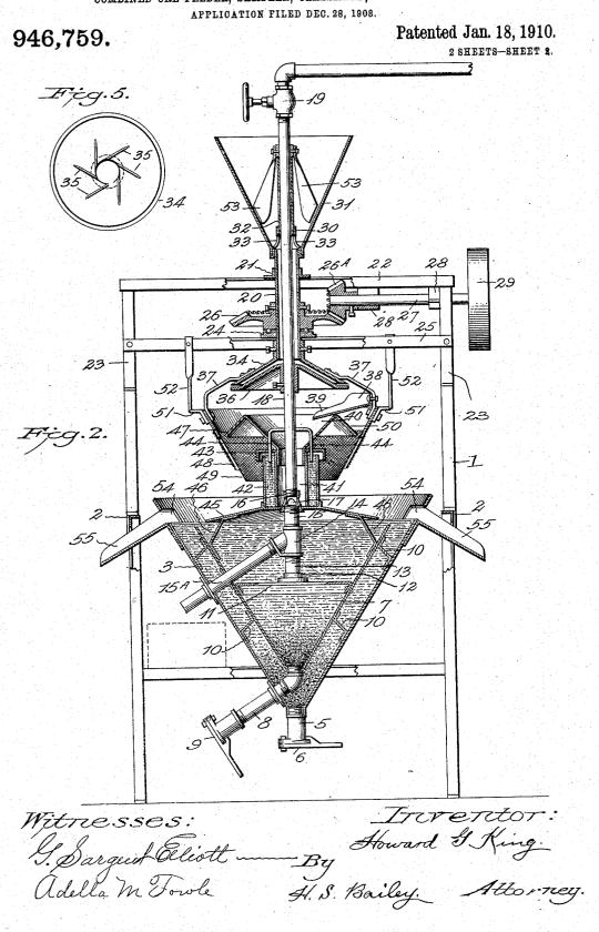
H. G. KING. COMBINED ORE FEEDER, SAMPLER, CLASSIFIER, AND SEPARATOR. APPLICATION FILED DEC. 28, 1908.
