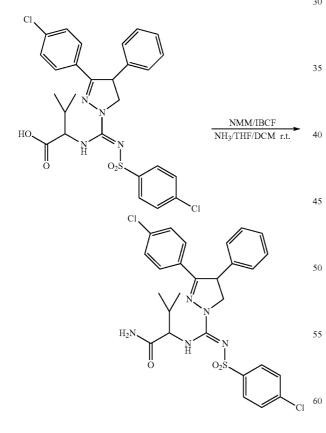
The L-valine adduct 21.4 g (37.3 mmol, 1.0 e.q.) in dichloromethane (DCM) (150 mL) containing N-methylmorpholine (NMM) 13.191 g (131 mmol, 3.5 e.q.) was mixed and 65 cooled to -10° C. A solution of isobutyl chloroformate (IBCF) 5.604 g (41.1 mmol, 1.1 e.q.) in DCM (50 mL) was
