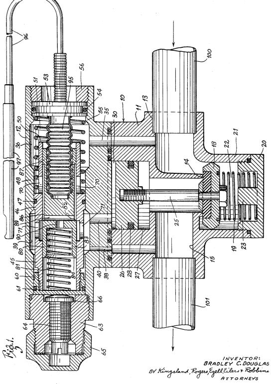
TEMPERATURE PILOTED EVAPORATOR PRESSURE CONTROL
