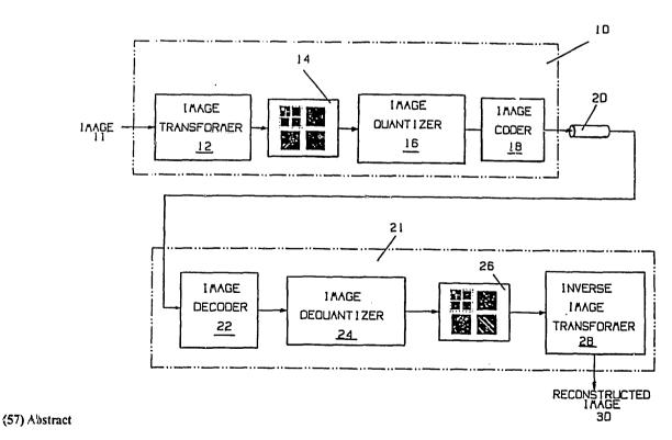
A system (10) compressing images is disclosed. The system utilizes a transformation (12) which is equivalent to expanding the image using a system of wavelets having finite support.
