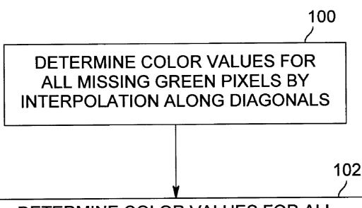
**DETERMINE COLOR VALUES FOR ALL** MISSING RED AND BLUE PIXELS FROM THE SUM OF AN INTERPOLATION TERM AND A LUMINANCE CORRECTION TERM BASED ON THE DIFFERENCES BETWEEN **VALUES OF GREEN PIXELS**
