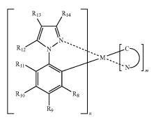
wherein at least one of  $R_8$  to  $R_{14}$  is phenyl or substituted phenyl, and/or at least two of  $R_8$  to  $R_{14}$  that are adjacent are part of a fluorenyl group. The emissive materials have enhanced electroluminescent efficiency and improved lifetime when incorporated into light emitting devices.
