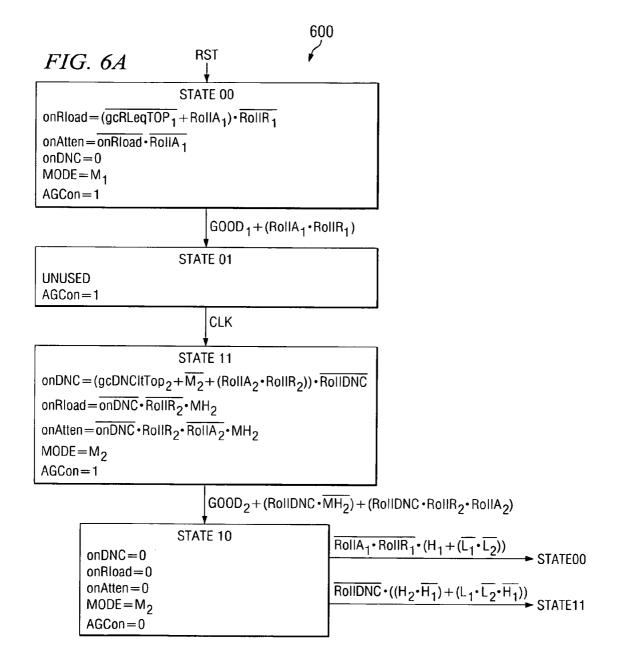
INPUTS: H<sub>1</sub>=TRUE IF PD1out>V<sub>H</sub>. THE SAME APPLIES TO MH<sub>1</sub>, M<sub>1</sub>, ML<sub>1</sub>, AND L<sub>1</sub>
