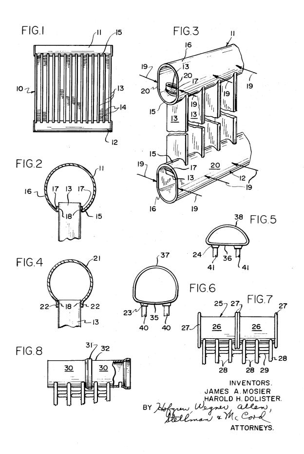
METHOD OF FABRICATING A HEAT EXCHANGER
