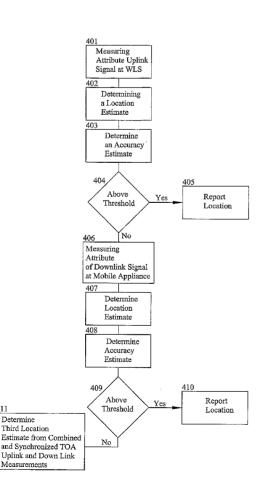
(57) Abstract: A method for use in a wireless communication system with a network overlay geolocation system having a sparse deployment network in which base stations of the wireless communication system may or may not have a co-located wireless location sensor (WLS). The method uses U-TDOA measurements on the uplink (reverse) signal and E-OTD measurements on the downlink (forward) signals to estimate a location for a mobile appliance.
