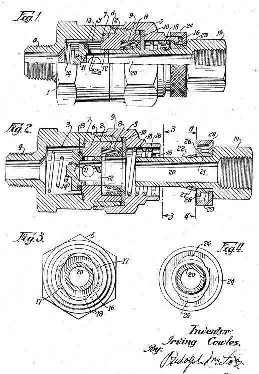
SEPARABLE SWIVEL CONNECTION FOR CONDUITS
