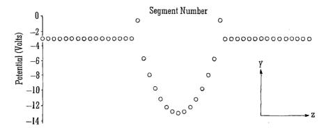
(57) **Abstract:** An ion trap mass analyser (1) is disclosed comprising a segmented rod set. Ions are trapped radially within the mass analyser by a radial pseudo-potential well. The ions are also confined axially within a quadratic axial potential well. A supplemental AC voltage or potential is applied to the electrodes comprising the ion trap mass analyser (1) in order to excite parametrically ions within the ion trap (1).
