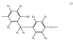
(wherein  $R_1$ ,  $R_2$ ,  $R_3$ , and  $R_1$  have the same meanings as defined above in the formula (1)) is less than 0.01 per 100 phenylene ether units of the formula (1). The resin has sufficient functionality and is well balanced between color tone/appearance and heat resistance/mechanical physical properties.
