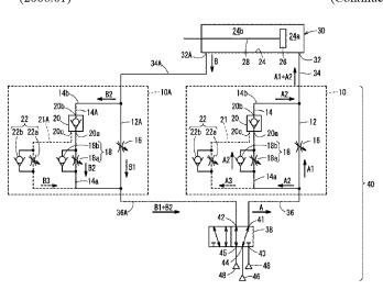
connected in series to the pilot check valve at a point along the second flow passage; a pilot air flow passage, one end of which communicates with the operation switching valve and the other end of which is connected to a pilot port of the pilot check valve; and a third flow rate adjustment part provided in the pilot air flow passage.
