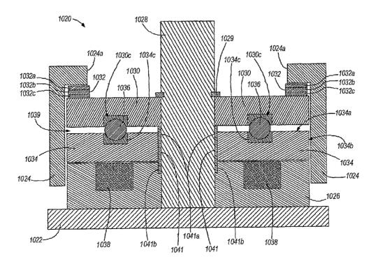
(57) Abstract: Residual magnetic locks, brakes, rotation inhibitors, clutches, actuators, and latches. The residual magnetic devices can include a core housing and an armature. The residual magnetic devices can include a coil that receives a magnetization current to create an irreversible residual magnetic force between the core housing and the armature.
