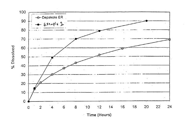
Figure 3. Dissolution Profile of Sodium Valproate XT Tablets, 576 mg and Depakote® ER Tablets, 500 mg in pH 7.5 Phosphate Buffer (Basket method at 100 rpm).
