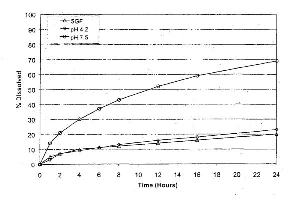
Figure 4. Dissolution Profile of Depakote® ER, 500 mg in SGF, pH 4.2 Acetate Buffer and pH 7.5 Phosphate Buffer (Basket method at 100 rpm).
