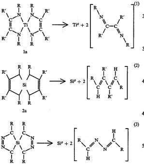
By the above processes, elemental titanium or silicon is deposited atop the wafer. The illustrated ligands which are oxidized from the precursor compound result in gaseous molecules having all atoms in a closed shell, non-ionic configuration, which are subsequently expelled from the reactor.
