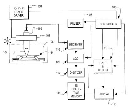
(57) Abstract: For use in acoustic micro imaging, a method (and implementing apparatus) is disclosed for creating a 4D virtual sample data memory (114). The method comprises employing a pulsed ultrasonic microscope probe (102) to interrogate a sample (94) at three-dimensionally varied locations in the sample (94). Data developed by the microscope probe (102) includes for each location interrogated a digitized A-scan for that location. The developed data is stored in a data memory (114).
