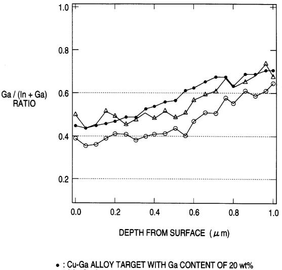
(1), Cu-Ga ALLOY TARGET WITH Ga CONTENT OF 20 wt% (2), AND In TARGET (3).
