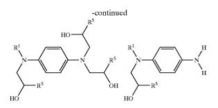
[0061] The reaction of 1,4-phenylenediamine with propylene oxide will also produce a mixture of products which include N,N'-dihydroxypropylphenylenediamine, N,N-dihydroxypropylphenylenediamine, N-hydroxypropylphenylenediamine, N,N,N'-trihydroxypropylphenylenediamine, and N,N,N',N'-tetrahydryoxypropylphenylenediamine.
